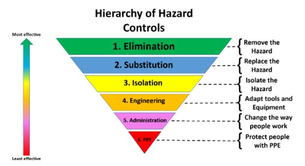
Figure 2. Hierarchy of Controls Pyramid.
